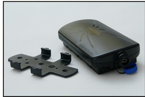
Secure the spider to the dashboard with the bracket supplied. The spider unit can be quickly removed from the mount when required. The top of the spider should point upward.
